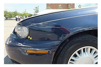
*Figure 3* - View of scuffs/scratches resulting from a vehicle-to-vehicle sideswipe contact.
