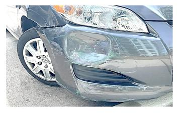
**Figure 1** - View of the excessive paint transfers that result from contact with a painted stationary object such as a wall/pole.
