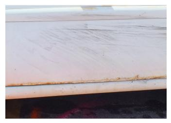
**Figure 4** - View of rotational tire marks resulting from a vehicle-to-vehicle sideswipe collision.
