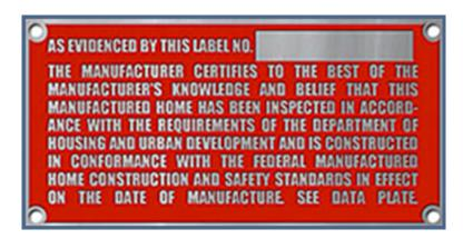
Figure 6 - Example of a mobile home certification label
