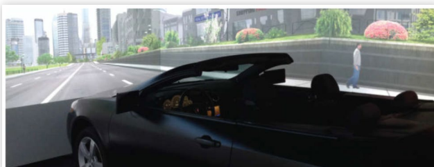
FIGURE 1 University of Guelph Driving Research in Virtual Environments (DRIVE) Lab full car Oktal driving simulator.
