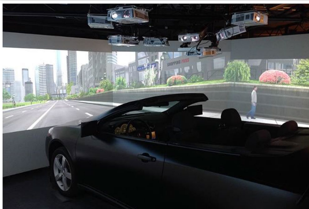
FIGURE 1 University of Guelph Driving Research in Virtual Environments (DRiVE) Lab full car Oktal driving simulator.
