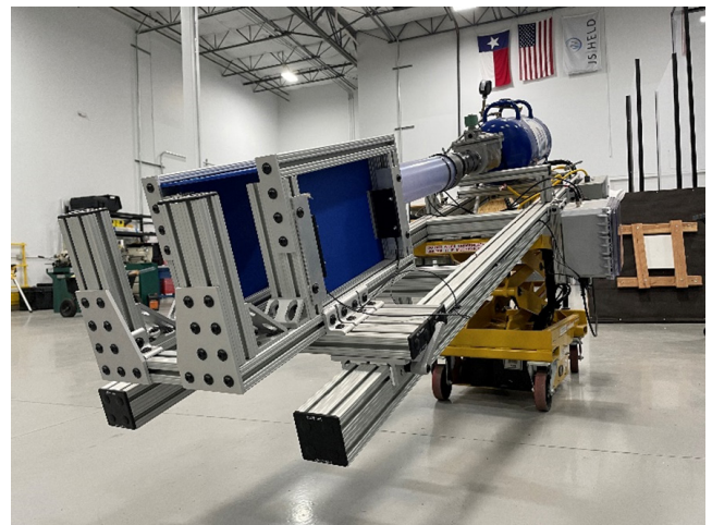
Figure 12 - Ice ball cannon, equipped with sophisticated timer and sensors for effective measurements of ice ball speeds.
