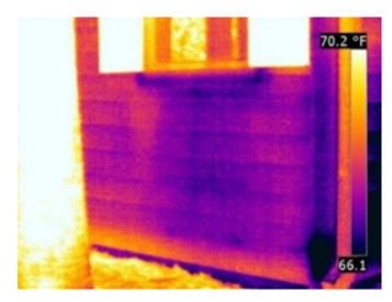
Figure 5 - Thermal anomalies below window
