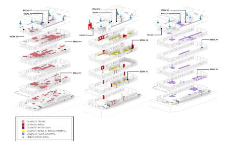
*Figure 3* - Water damage project, animation representing sequence of pipe breaks, affected elements, and quantification of the damages.
