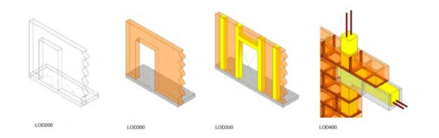
Figure 1 - BIM Levels of Development (LOD) / Levels of Information. Masonry wall element progression.
