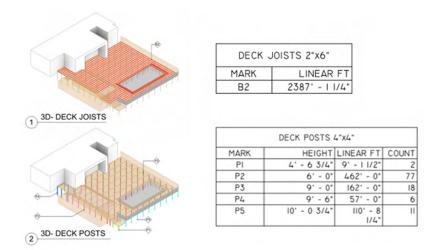
Figure 6 - Lims model reflecting spreadsheet data for deck joists and posts.
