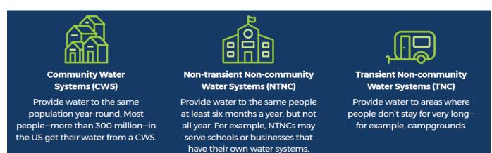
Figure 1 - U.S. public water system types (Source: EPA).
