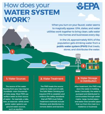
Figure 2 - How public water systems work (Source: EPA).
